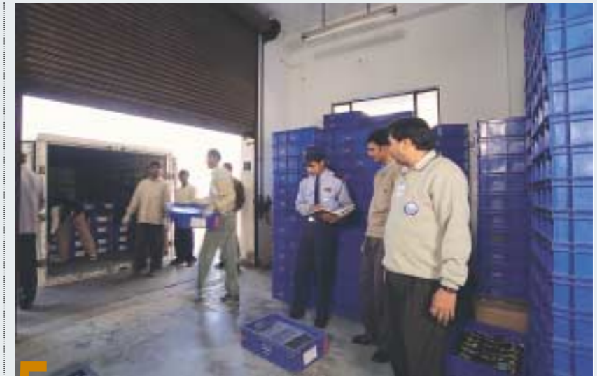
5 Dispatch: Under MUL's e-nagara system, delivery is done once/twice/multiple times in a day. Loading is done using the Last In First Out principle.
