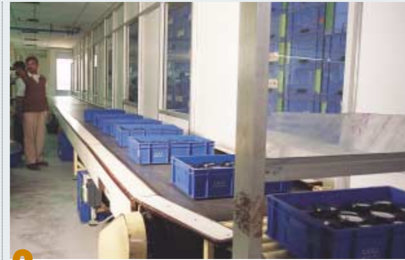
3 Packing: Components are put in specified bins, labeled and sent to MUL. Saves costs for vendors within 200 km radius. Cost rises beyond 200 km radius, as packing needs to be done twice.
